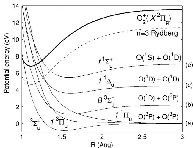
FIG. 1. Schematic of the diabatic potential curves relevant for the DR of  $O_2^+$ . The dissociation limits connected with each valence capture state are given on the right. The labels (a)–(c), and (e) refer to Eqs. (1a)–(1c) and (1e), respectively.
