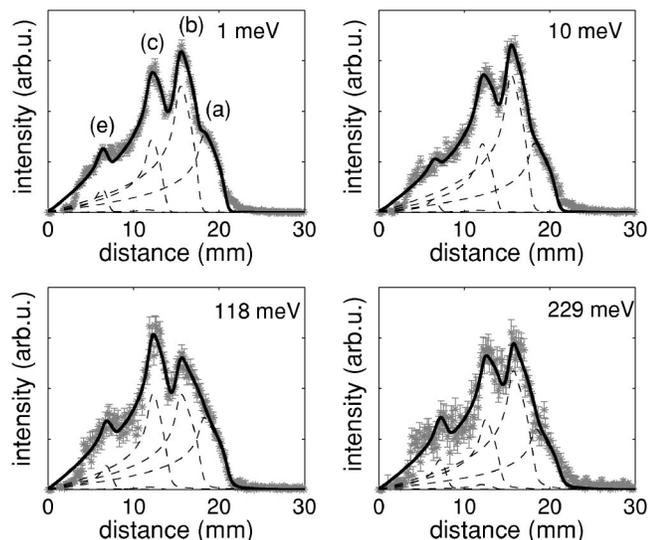
FIG. 2. The distance distributions of the DR of  $O_2^+$  at collision energies of 1, 10, 118, and 229 meV (space-charge corrected energies). The stars are the experimental data and the solid curves are the simulations based on isotropic distributions. The peaks corresponding to the dissociation limits given in Eqs. (1a)–(1c) and (1e) are indicated at 1 meV with the labels (a)–(c) and (e), respectively. The dashed lines show the contributions of the dissociation limits as results from the fits.
