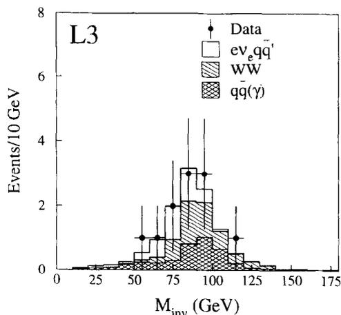
Fig. 7. The jet-jet invariant mass spectrum,  $M_{\text{inv}}$  of the selected hadronic candidates for the combined data sample. The hatched histogram represents the background, the open histogram shows the fitted signal from  $e^+\nu_e q\bar{q}'$  final states.
