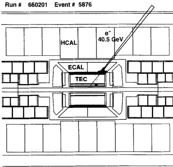
Fig. 4. A  $e^+e^- \rightarrow e^+\nu_e W^-$ ,  $W^- \rightarrow e^-\bar{\nu}_e$  candidate event. In the upper hemisphere the 40.5 GeV electron is detected in the tracking chamber and in the electromagnetic calorimeter where the pulse heights represent the electron energy deposition. No significant energy deposition is observed in other subdetectors since the positron escapes in the beam pipe.
