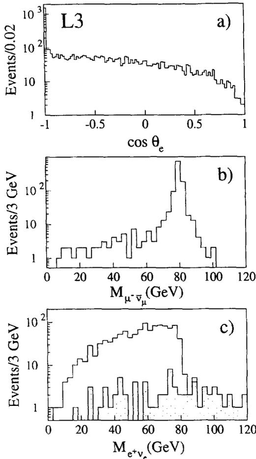
Fig. 2. (a) The positron polar angle spectrum for all  $e^+ \nu_e \mu^- \bar{\nu}_\mu$  final states generated by GRC4F at  $\sqrt{s} = 161$  GeV. The invariant mass spectrum of the  $\mu^- \bar{\nu}_\mu$  (b) and  $e^+ \nu_e$  (c) pairs for the events satisfying phase space conditions (2). The hatched histogram in (c) represents events which meet the requirement  $|M_{\mu\bar{\nu}_\mu} - M_W| > 10$  GeV.
