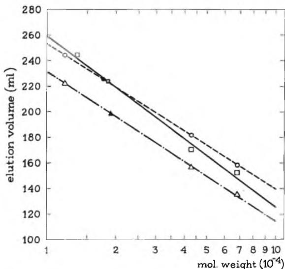
Fig. 2. Graphical interpretation of elution data of separated fractions from a Sephadex G-100 column equilibrated with 6 M urea-0.05 M phosphate buffer at pH 7.6. — ○ — serum albumin, ovalbumin, cytochrome c and CM- $\alpha$ ; — △ — serum albumin, ovalbumin, cytochrome c and CM- $\alpha_1$ ; — □ — serum albumin, ovalbumin, ribonuclease and CM- $\alpha_2$ .
