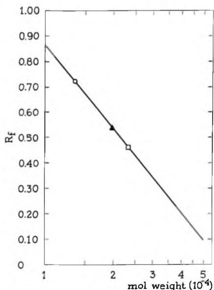
Fig. 4b. Graphical interpretation of the electrophoretic migration data of the different proteins shown in fig. 4a.  $\circ$  RNase;  $\blacktriangle$  CM- $\alpha$ A<sub>1</sub>;  $\square$  trypsin.
