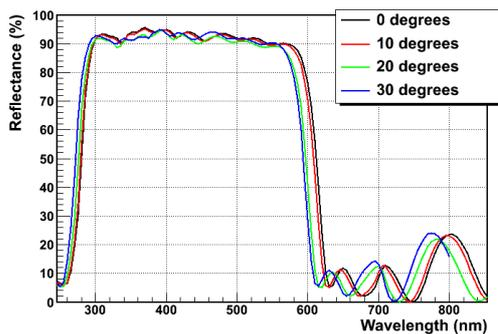
Figure 5: Simulated reflectance vs. wavelength of the above-described 28-layers  $TiO_2$ - $SiO_2$ - $HfO_2$  coating design, at different incident angles (0 degrees corresponds to normally incident light).
