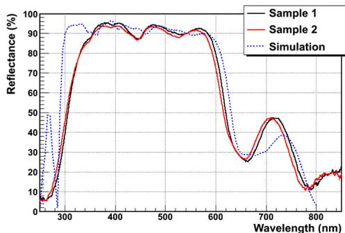
Figure 3: Measured reflectance vs. wavelength for normally incident light on a 24-layers  $\text{TiO}_2$ - $\text{SiO}_2$  coated glass substrate (red and black line) and simulation (blue dashed line). The reflectance was measured with an Ocean Optics JAZ hand reflectometer, kindly provided by MPIK Heidelberg.
