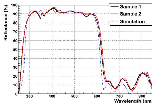
Figure 4: Measured reflectance vs. wavelength for normally incident light on a 24-layers  $\text{TiO}_2$ - $\text{SiO}_2$  plus 4-layers  $\text{HfO}_2$ - $\text{SiO}_2$  coated glass substrate (red and black line) and simulation (blue dashed line). The reflectance was measured with an Ocean Optics JAZ hand reflectometer, kindly provided by MPIK Heidelberg.
