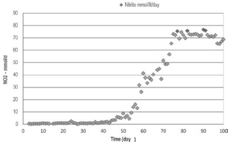
**Figure 4.** Nitrite conversion during the experiment. Through 0 to 40 day period consumption fluctuates from 0.6 to 4 mM (not displayed in the graph), after 40 days the growth of anammox is exponential and by day 80 consumption stabilizes.
